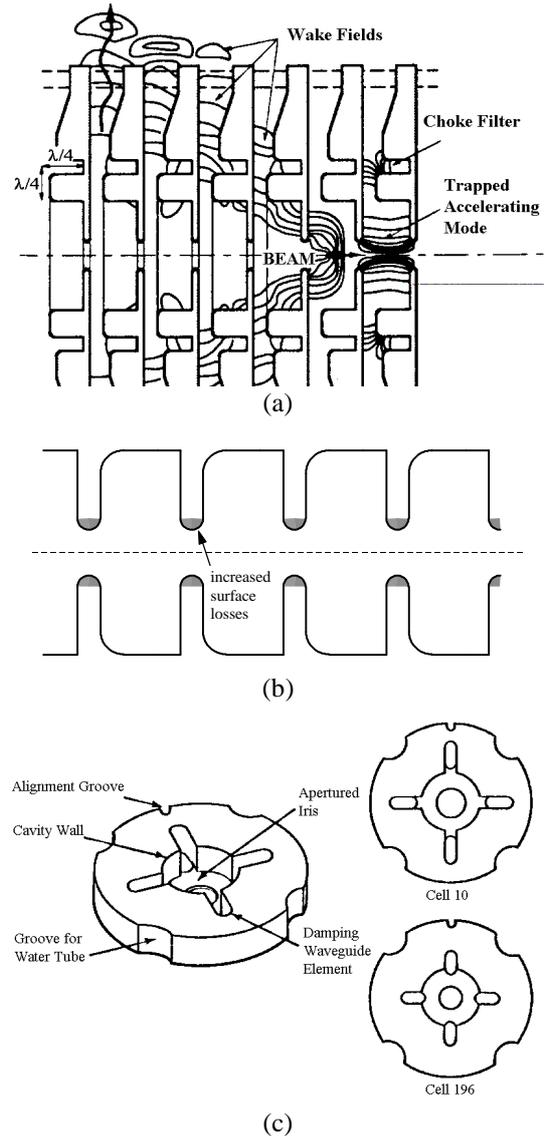
Fig. 3. Damped structures: a) Concept of the HOM-free choke mode accelerating structure. b) Manifold damped structure. c) Damping by increased losses on the iris lip.
