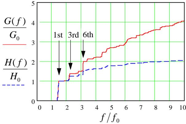
Fig. 1. Normalized sum of loss- and kick-parameters,  $G_0 = G(1.5f_0)$ ,  $H_0 = H(1.5f_0)$ .
