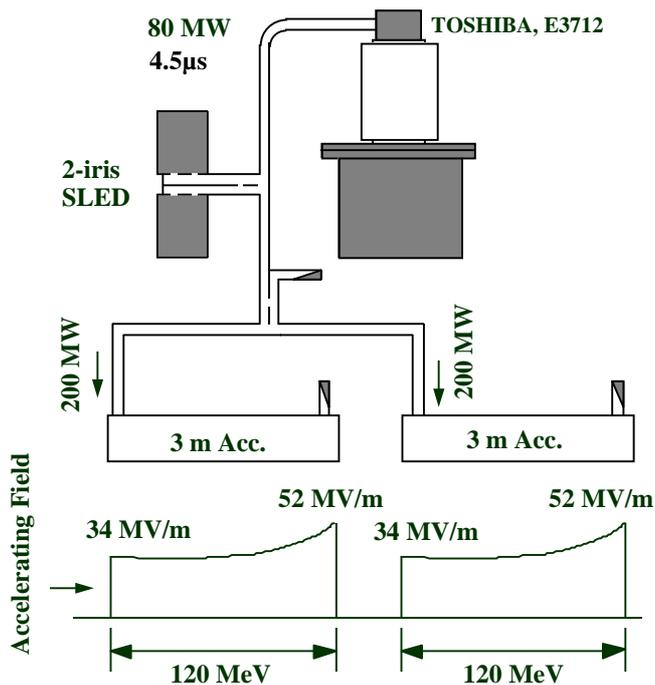
Fig. 1. Block diagram of the high gradient accelerating unit.
