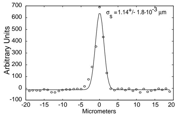
Figure 4. A typical profile monitor scan showing  $\sigma_{sy}$ . The horizontal scale is determined using the transfer matrix ( $R_{34}$ ) for the scan coils to the laser IP. The collision signal in this case is detected using the SLD polarimeter degraded e- detector, located after the first large bend in the outgoing beamline. Each data point is the average of 3 beam pulses with the laser on, with the average of 6 pulses with the laser off subtracted.
