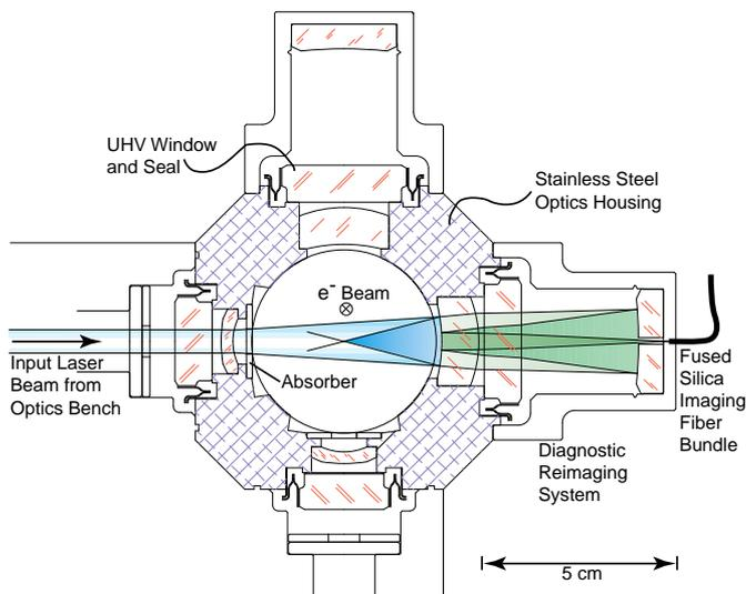
Figure 2. Central cross section of IP Optics. The parallel laser beam ( $z_R \gg 20m$ ) enters at right or from underneath with a  $\sigma_{in}$  of about 2.5mm. The four 8mm thick UHV seal windows with their weld rings are placed on each side of the IP, with the precision optics installed inside the vacuum chamber. 1% of the light is transmitted and re-imaged on the far side of the IP for diagnostic purposes.
