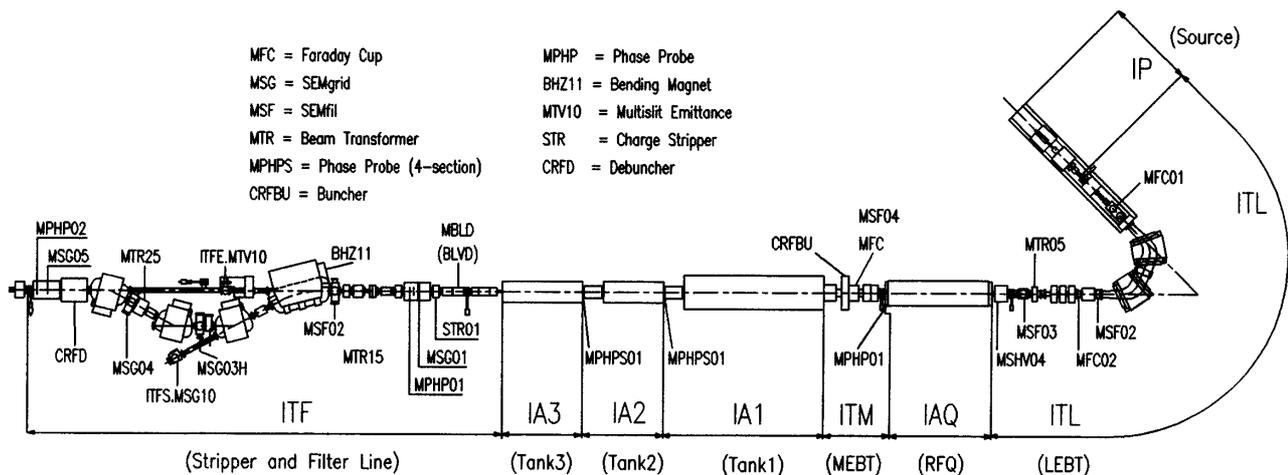
Fig.2 Layout of Linac3 with filter line
