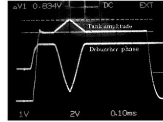
Fig. 4: Debuncher phase (lower), tank 3 amplitude (upper trace)
