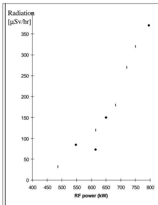
Fig. 3. Radiation levels near tank 2
