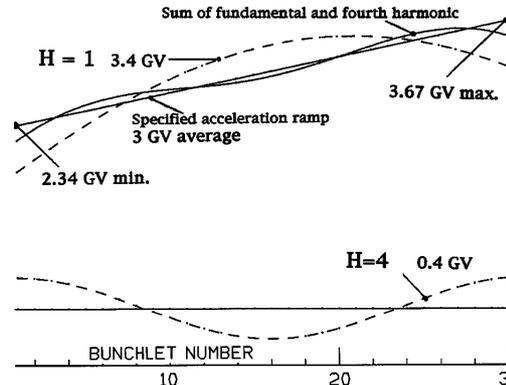
Fig. 3. Acceleration ramp synthesis.
