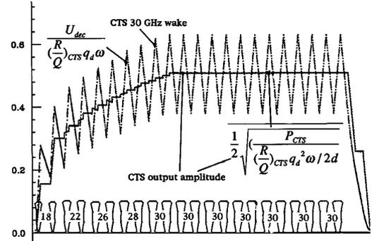
Fig. 2. Computer optimized bunchlet numbers, relative intensities, normalized 30 GHz CTS wake amplitudes (dashed, linear variations of  $\pm 23\%$ ) and the normalized CTS output amplitude.
