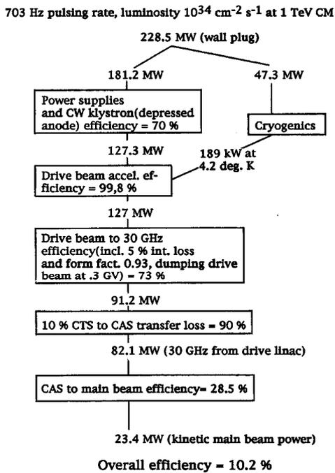
Fig. 6. Wall plug to main beam efficiency.
