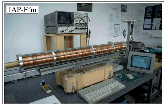
Fig. 2: Measurement setup with 36-cell structure
