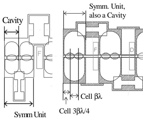
Figure 1. Cell, cavity, and symmetric unit in a 1- and 2-drift-tube CCDTL.
