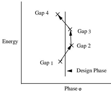
Figure 2. PARMILA adjusts the symmetric unit length and the entry phase until the design phase equals the average reference particle phase.
