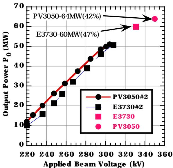
Fig. 3. Output-power characteristics as a function of the applied beam voltage
