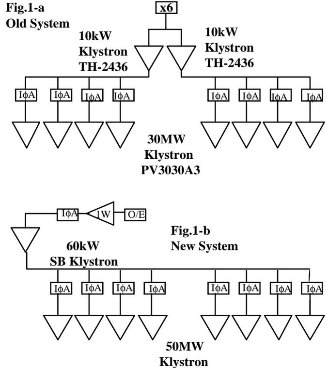
Fig. 1. Comparison between the old and new driving systems.
