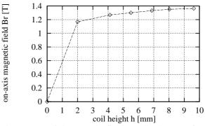
Figure 4. Radial magnetic field amplitude  $B_r$  as function of the coil height h with constant inner radius  $r_i$  of 2mm.
