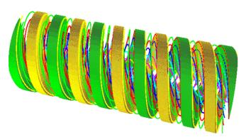
Figure 2 Solid model of the undulator as it is used in the numerical calculations with current filaments and iron between the conductors.
