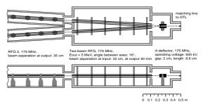
Fig. 11. Scheme of the ESS funneling section.
