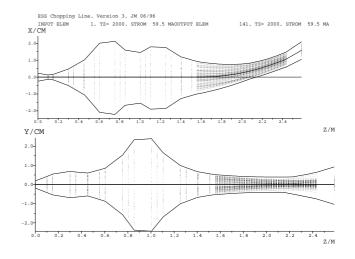
Fig. 7. Transversal behaviour of the chopped beam along the chopping line.
