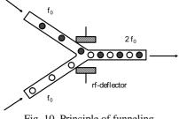
Fig. 10. Principle of funneling.
