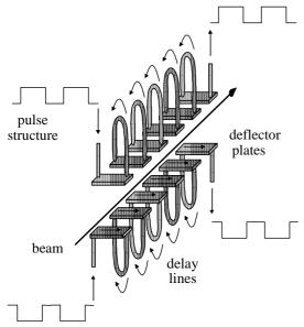
Fig. 3. Schematic drawing of the chopper structure.
