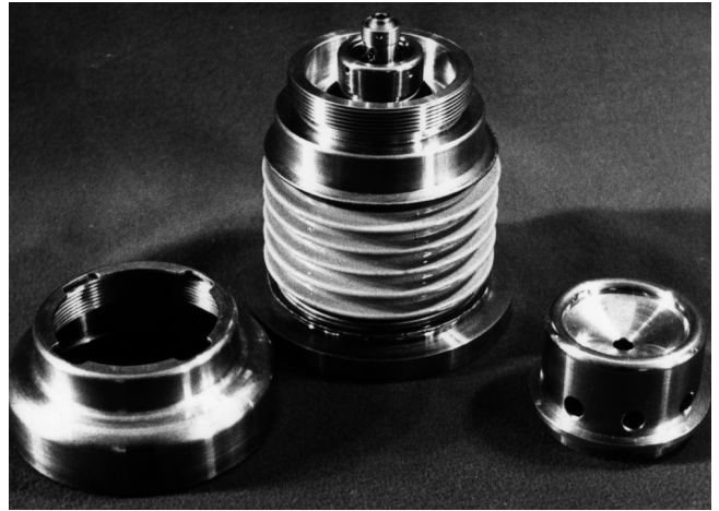
Fig.3. The main parts of electron gun high voltage assembly.
