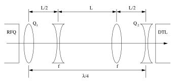
Fig. 1. The Brown-Servranckx matching transformer used to match a beam from an RFQ to a DTL.
